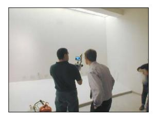
This process was monitored by infrared thermography done while the exothermic heat of the chemical reaction was present. This verified that the void was filled to the required level with the new insulation. This quality assurance procedure was video recorded as the work progressed.
