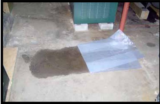
3. Remove the bag and see if the slab is wet. This indicates that the water vapor is migrating into the interior space from the ground
