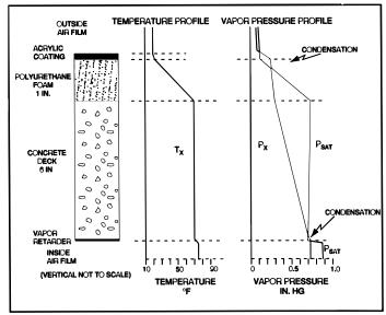
plane is due to water vapor diffusing up through the deck and polyurethane foam and reaching a temperature below the dew point. Corrective action would be the installation of a vapor retarder on the bottom of the deck.
